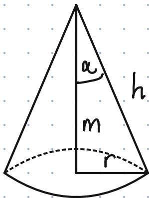
$$\left. \begin{array}{l} V = \frac{1}{3} r^2 \pi m \\ r = h \sin \alpha \\ m = h \cos \alpha \end{array} \right\} \begin{array}{l} V(\alpha) = \frac{\pi}{3} h^2 \sin^2 \alpha h \cos \alpha \\ V(\alpha) = \frac{\pi}{3} h^3 \sin^2 \alpha \cos \alpha \end{array}$$
